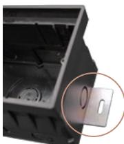
There are two metals support plate on the bottom of the sleeve. It is used for fixing and preventing the mounting sleeve shifting while filling the concrete.
